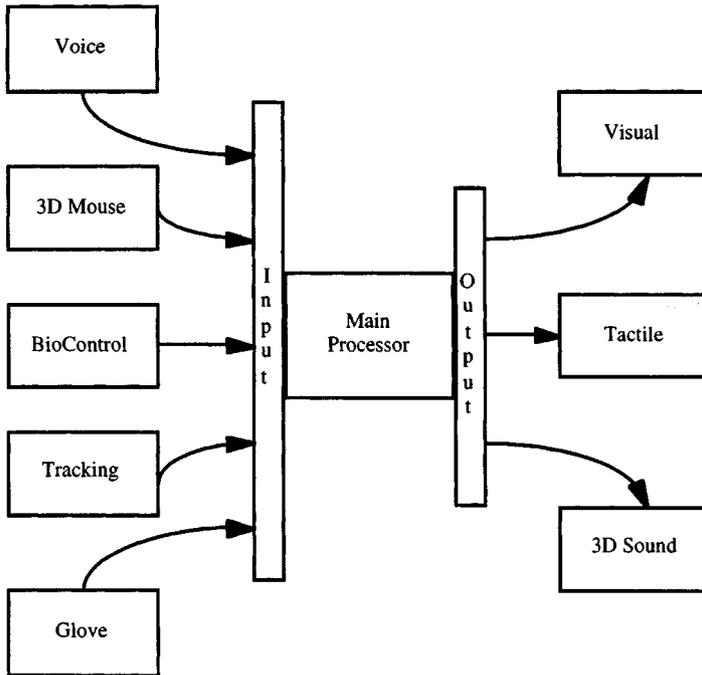
Fig. 14.1 Hardware in a VR system.
