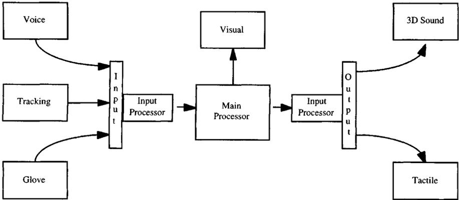
Fig. 14.2 VR system architecture.
